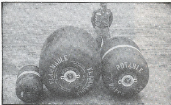
Rajah 9: Tiga saiz APFC. Di kiri berukuran 28 liter/55 gelen, di tengah 2250 liter/500 gelen dan di kanan 1125 liter/250 gelen. (Plate 9)
