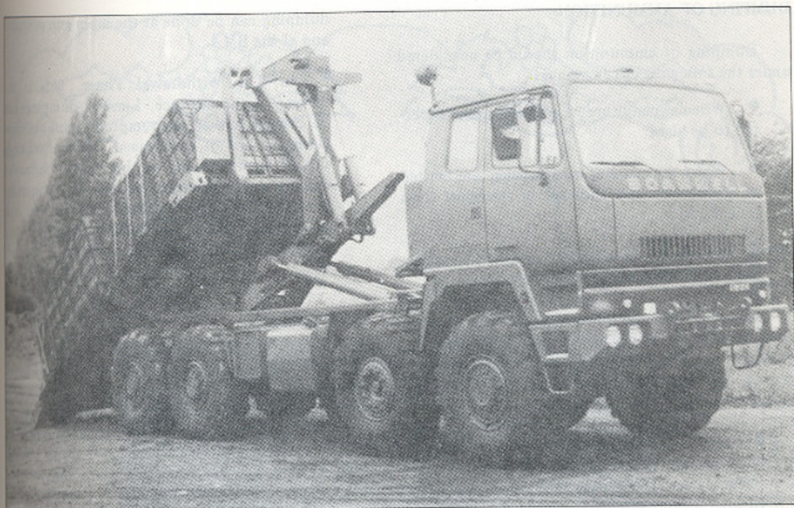
Unloading ammunition from a carrier fitted with a hydraulic power system
