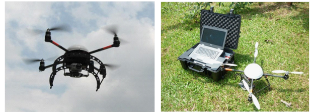
Figure 2: Helicopter type UAV and its ground control system.
