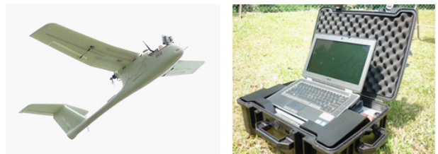
Figure 3: Small fixed wing UAV and its ground control system.
