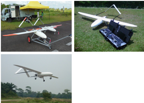
Figure 4: Medium fixed wing UAV and its ground control system.
